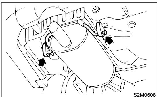
3) Remove front rubber cushion, and detach muffler assembly.
