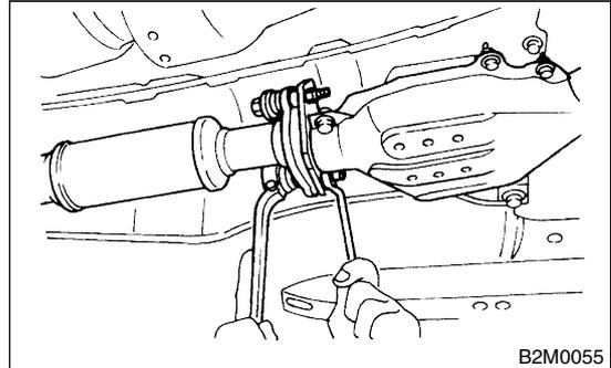
6) Tighten bolt which holds front and center exhaust pipe assembly to hanger bracket.
