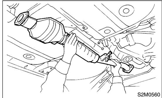
2) Install rear exhaust pipe to muffler.
