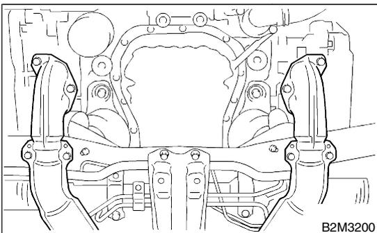
5) Tighten bolts which install front and center exhaust pipe assembly to rear exhaust pipe.
