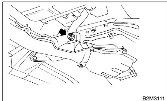
7) Install under cover. <Ref. to EI-11, INSTALLATION, Front Under Cover.>
