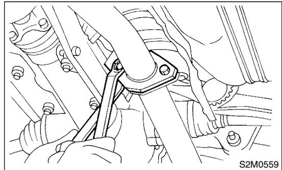
3) Install rear exhaust pipe to center exhaust pipe.
