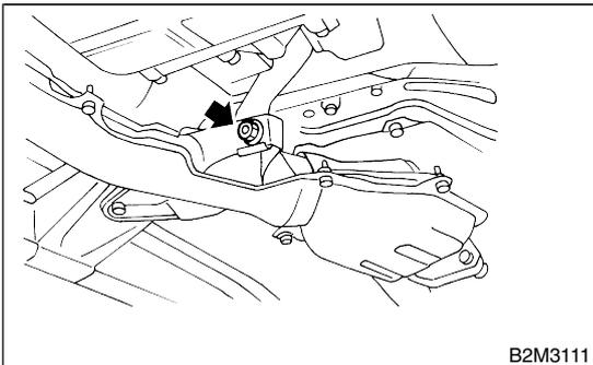
4) Tighten bolts which hold front exhaust pipe onto cylinder heads.
