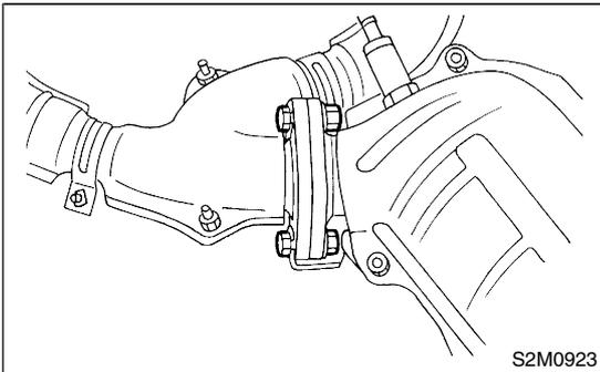
2) Install front and center exhaust pipe assembly to the vehicle.
