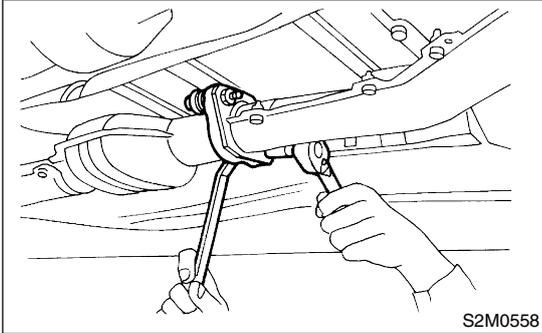
2) Separate rear exhaust pipe from muffler.
